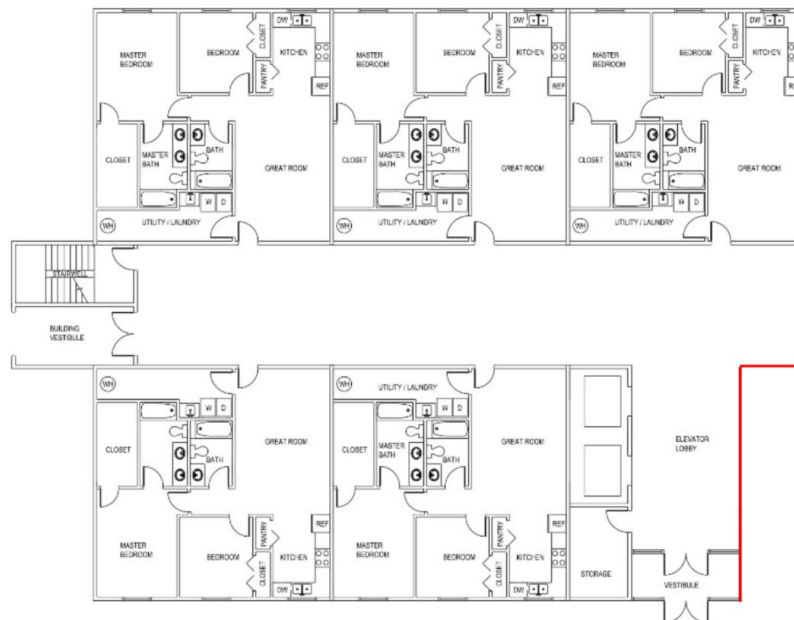
Figure 5: 45-Unit Multifamily Residential Floor Plan – West Side
