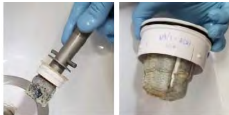
Figure 4 - Sumplex Cartridge Style with Silicon Check Valve (1 Month Operation)
