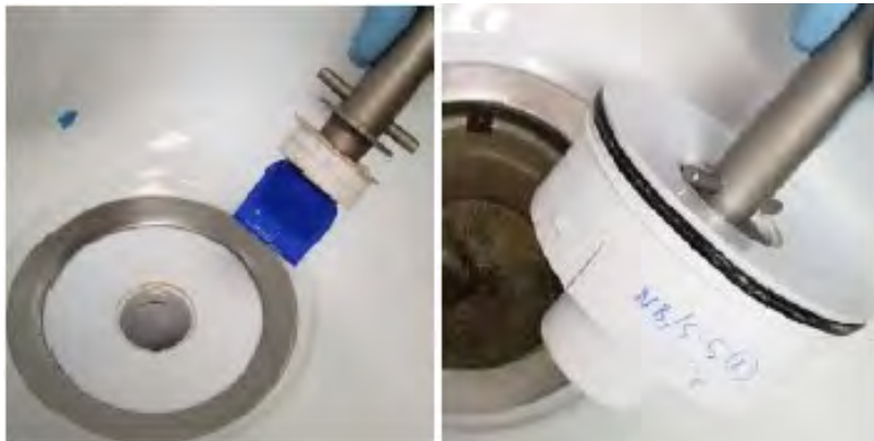
Figure 3 - Sumplex Cartridge Style with Silicon Check Valve (2 Months Operation)
