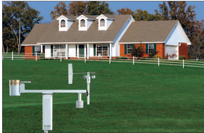
Above: Weather station monitors and stores daily evapotranspiration (ET) parameters, including air temperature, solar radiation, relative humidity, wind speed and rainfall.
